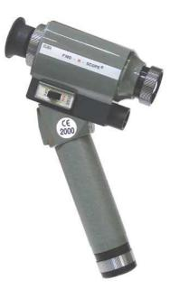
The FIND-R-SCOPE 85100-5 is a self-contained, hand-held Infrared Viewer with a built-in LED Illuminator, an extended spectral sensitivity of 350-1550 nm, and optional C-mount capability. Note: The 85100-5 replaces the discontinued model 85100A-5.
